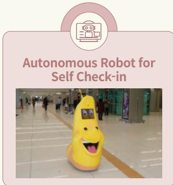
KAC introduced the "Autonomous Robot for Self Check-in" shaped like an animation character which issues boarding tickets when passengers input their registration number on touch screen. When meeting passengers, this robot is transformed into an automatic dispenser. Meanwhile, we integrated self-check-in systems which were independently managed by each airline into a common-use self-check-in system to increase space efficiency and ease congestion at terminal.
