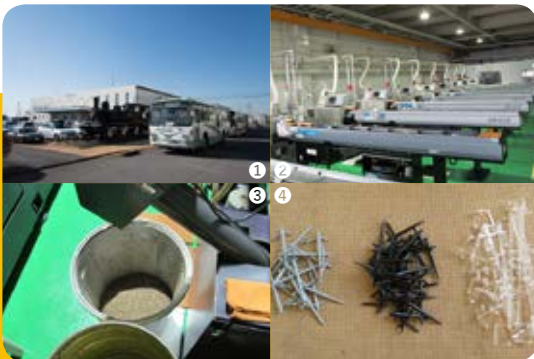
①TOMY TEC (Tochigi) ②Equipment that makes TOMIX train wheels ③Metal scraps left over after cutting train wheels are recycled ④Runners discarded during plastic molding
