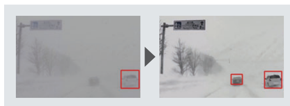
Technology to remove the effects of snow or fog for clearer images Before removal (Left) / After removal (Right)
