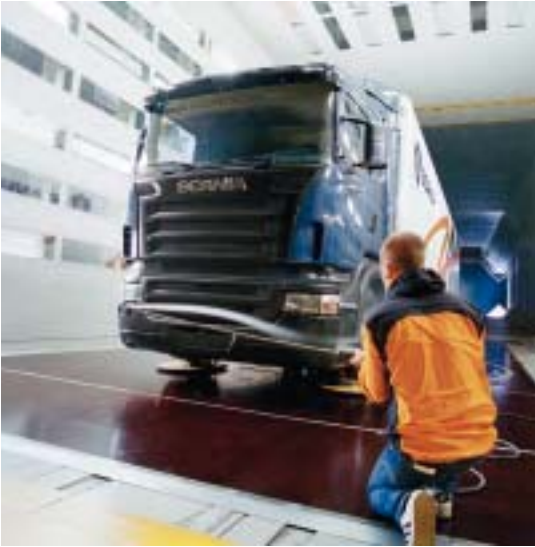
Different outer panels are tested in the wind tunnel to improve aerodynamics and reduce fuel consumption. Fuel-efficient driving is also guaranteed by the engines, which are equipped with the latest combustion technology.
