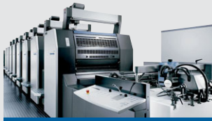
Sheetfed offset presses for 50 × 70 cm format (20 × 28 inches)
