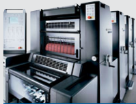
Sheetfed offset presses for 35 × 50 cm format (14 × 20 inches)
